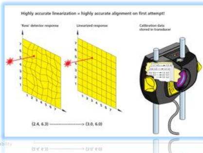
A calculation is then made by the shape of the ellipse to get misalignment readings for both shaft offset and angularity
