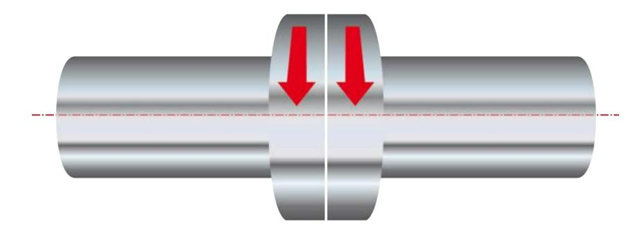
at the point of power transfer from one shaft to another, the axes of rotation of both shafts should be colinear when the machine is running under normal operating conditions
