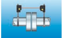
Laser-optical alignment Resolution 1/1000 mm
