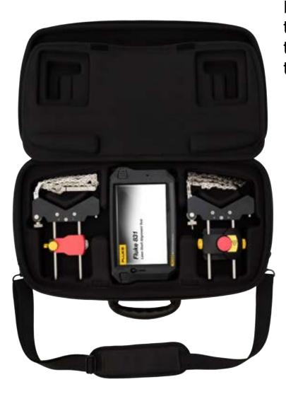
Mount the brackets on either side of the coupling on either the shafts or on the solid coupling hubs, and both at the same rotational position.
