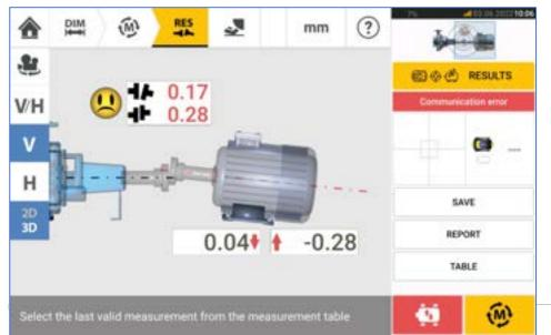
directly related to the coupling alignment condition as follows: **Blue** – excellent (foot should not be moved) **Green** – acceptable (if possible, foot should remain unaltered) **Red** – poor (foot requires moving to attain a better alignment condition)
