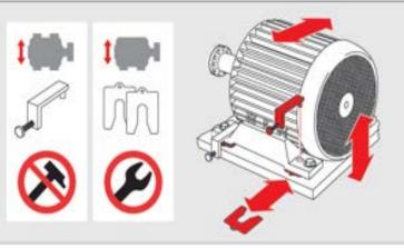
After moving machines to within tolerance, tighten the foot bolts then tap 💮 to remeasure.
