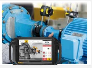
"We electricians would replace the motor bearings and mechanics would replace the pump bearings and seals, and we'd slap it all back together. In a few months we would do it all over again. Then we learned to perform precision shaft alignments, and the bearings would last for years and years." Maintenance Supervisor from US Navy
