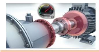
Flexible couplings do not make up for the misalignment in a machine they simply transfer the forces to the bearings and seals causing rapid wear and failure
