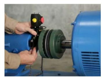
Mount Sensor on "Left machine" – usually Stationary
