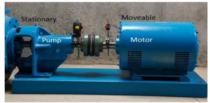
Typically: Mount sensor on "Left machine" – usually Stationary (pump) Mount prism on "Right machine" – usually Moveable (motor)
